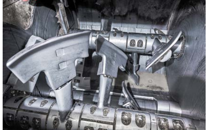
Twin-shaft mixer after the automatic cleaning with the Stetter HighEfficient Cleaning System
