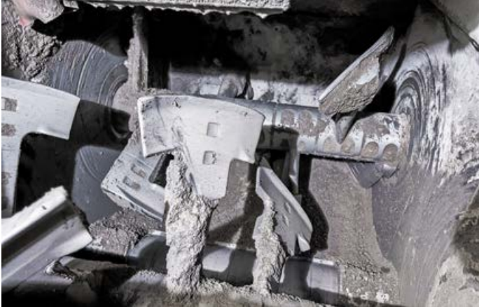
Twin-shaft mixer after the mixing process
